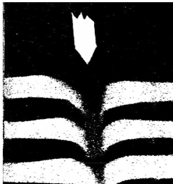
Figure 14: The disruption of the original structure of a mixture by a sample thief.
